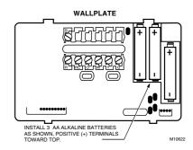
If the thermostat is already mounted on the wall, remove the thermostat by placing your thumb between the thermostat and wallplate and pulling the thermostat up and away as shown.
