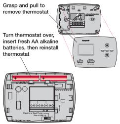
Install fresh batteries immediately when the **REPLACE BATT** warning begins flashing. The warning flashes about two months before the batteries are depleted.
